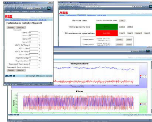
Fig. 7. Views of the different services: Top left shown is the configuration page of the measurement; top right the operational status of the device. On the bottom the output of a java applet is shown with the data of the temperature and gas flow controllers.
